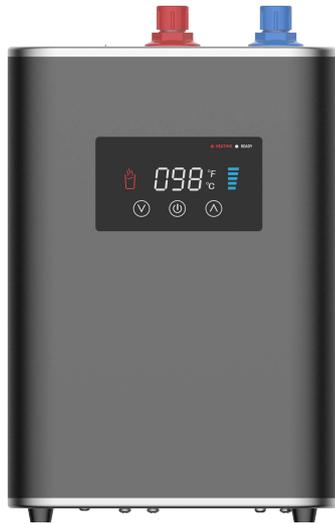
The hot water heater is open vented (non-pressured) and intended for Point-of-Use (POU) installation to connect one water outlet only. Only "Open Vent" faucets function with the hot water heater. Connecting a standard faucet will damage the heater and void the warranty.
