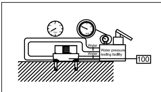
2. Make pressure test for the base union 100 by 10 hours in 10 bar to assure there is no any leakage before the next step.
