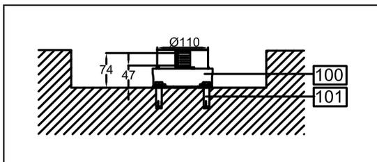
1. Mount the base union 100 onto the cement ground with 101 and keep it horizontal.
