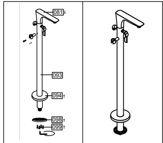
6. Put the covers 094 onto the pole 093 and mount the fixing round plate 098 onto the end of pole 093. Meanwhile fix the post 081 onto the body, locking with hexagonal spanner.
