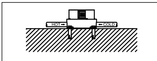
3. Connect the water inlets with the feeding pipes.
