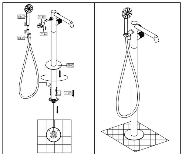
7. Take away the protective cover from the base union E190 and mount the poles E178 onto the base plate, locking with the nuts E192. Then slide down the cover E180 onto the floor.
