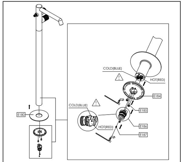
6. Put the covers E180 onto the pole E178 and mount the fixing round plate E184 onto the end of pole E178.
