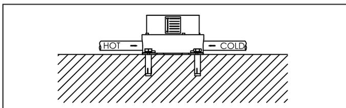
3. Connect the water inlets with the feeding pipes.
