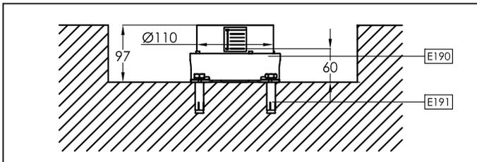
1. Mount the base union E190 onto the cement ground with E191 and keep it horizontal.
