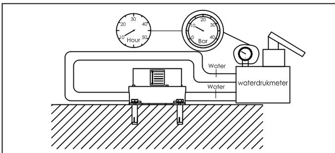
2. Make pressure test for the base union E190 by 10 hours in 10 bar to assure there is no any leakage before the next step.
